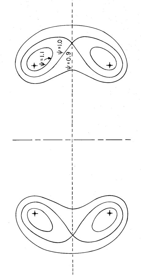
Figure 5 - Lines of constant magnetic pseudopotential for Helmholtz geometry.
